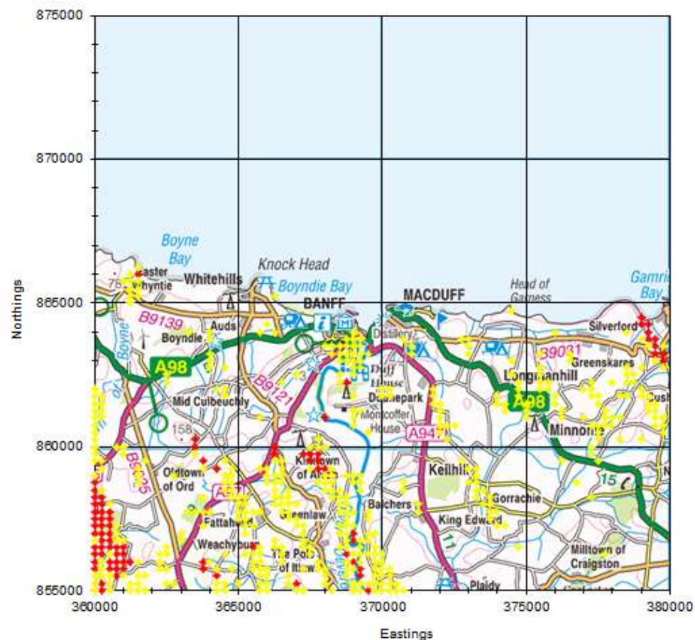
Figure 14 Interference map for the Rumster Forest TV Transmitter – 250m resolution – Area 2
