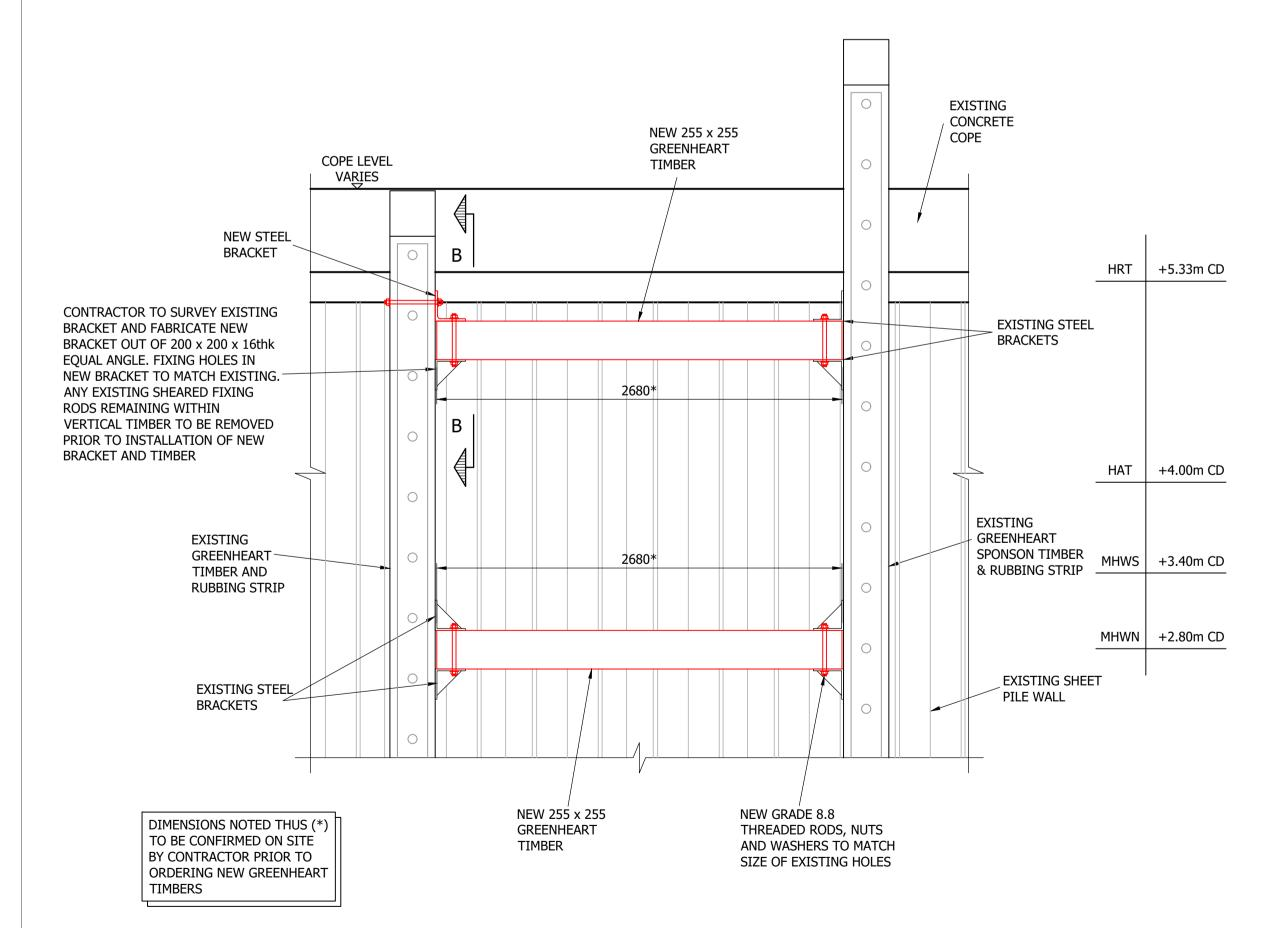
ELEVATION ON MISSING TIMBERS ch203 TO ch206 SCALE 1:25
