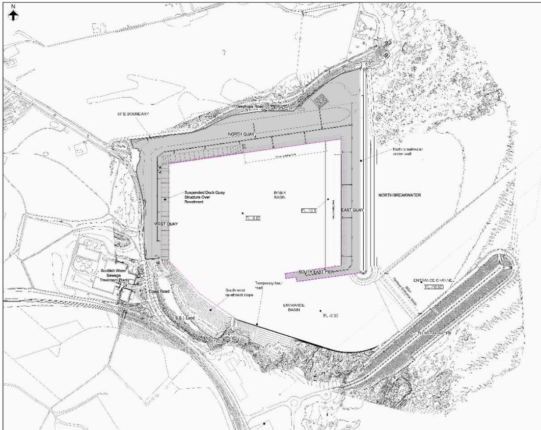
Figure 14.1: Layout of harbour showing the West and North Quay suspended decks
