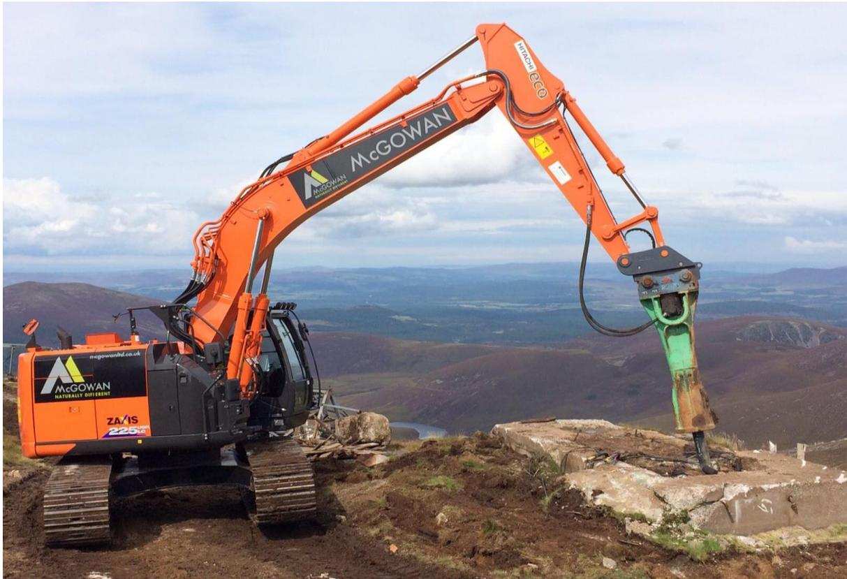
Excavator with Breaker Attached
