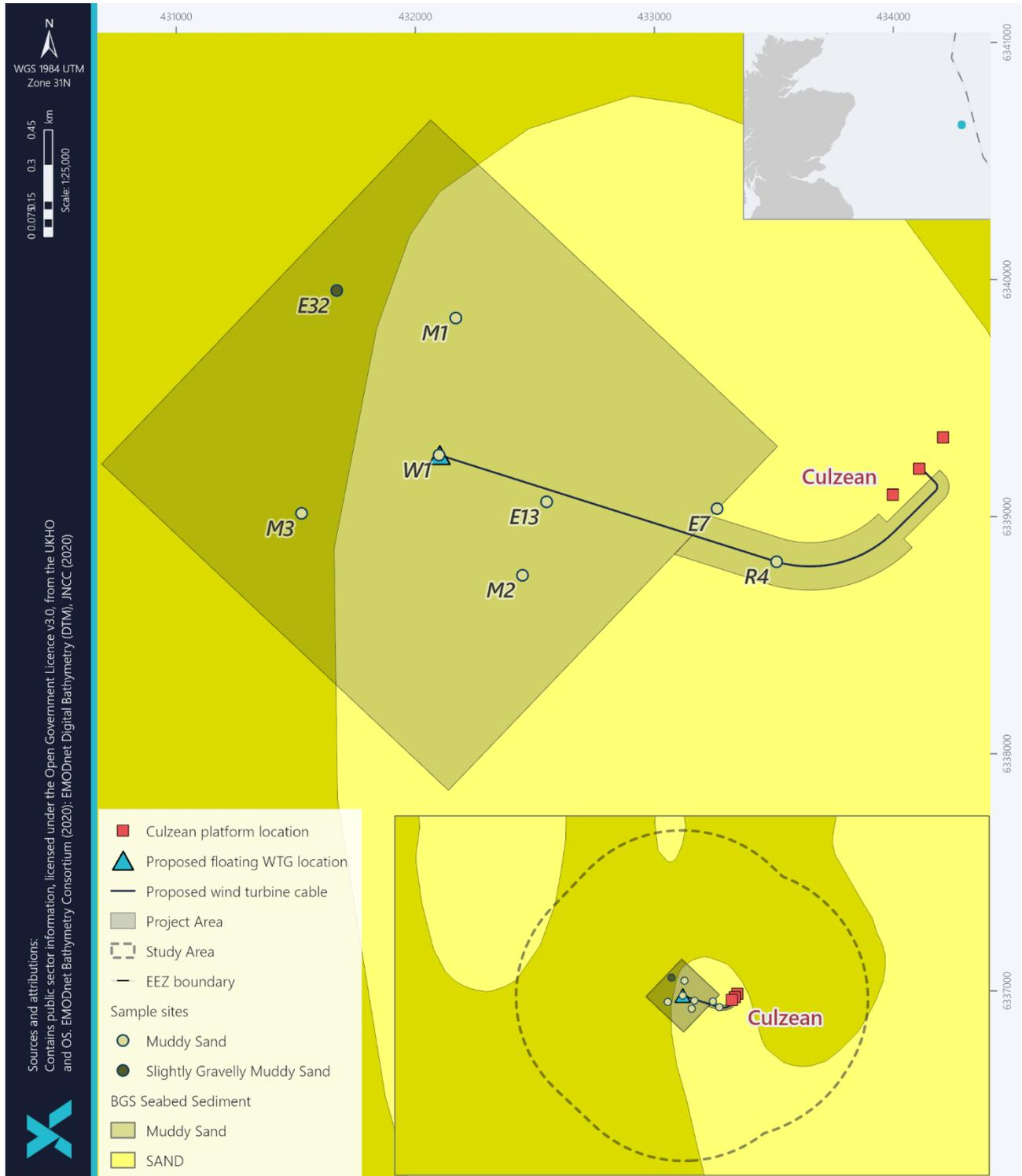
Figure 7-4 Sampled seabed sediment properties across the Project Area in relation to BGS (2023)
