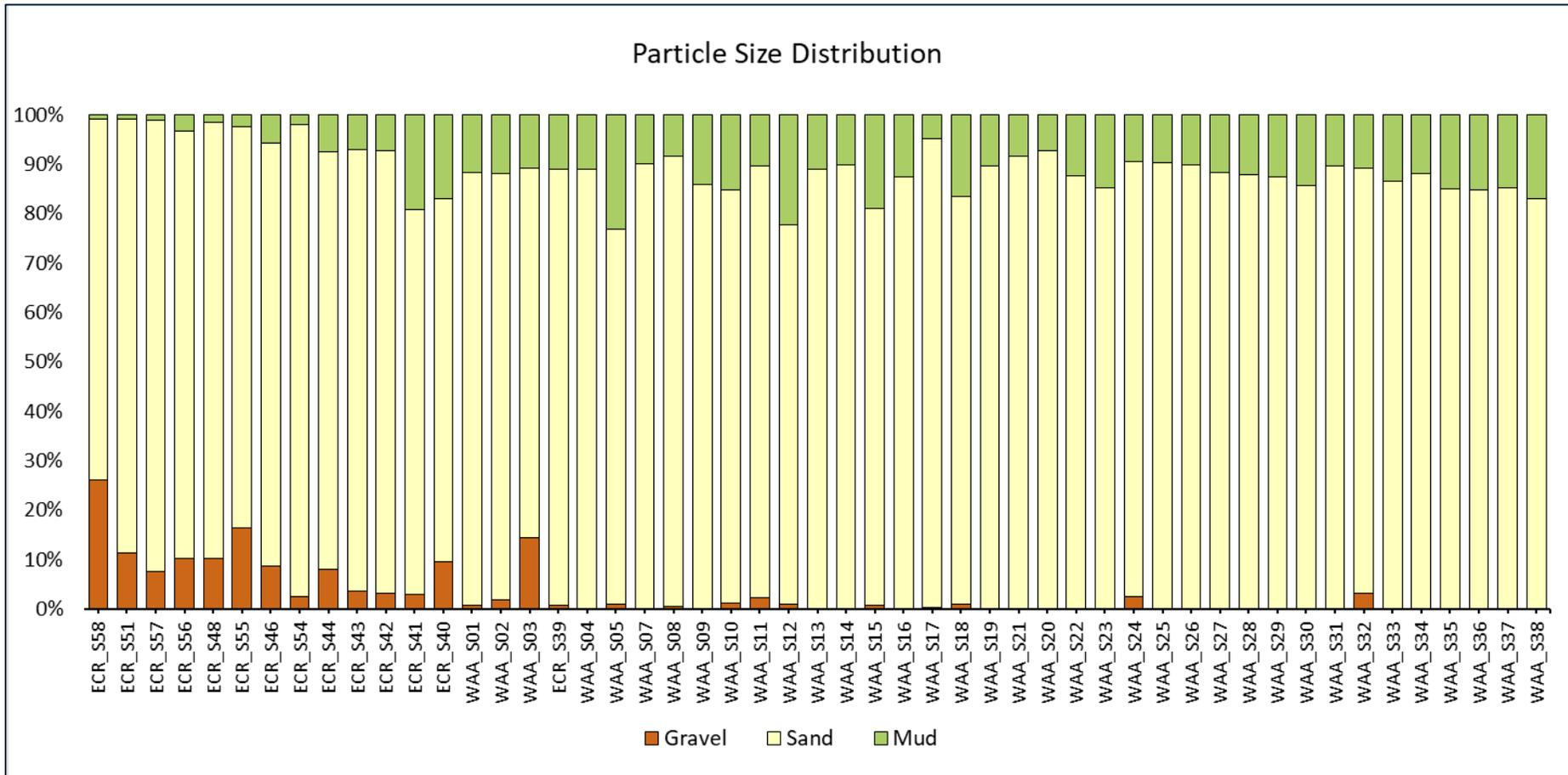
Figure 13 Particle size distribution from grab samples, sorted by increasing easting.
