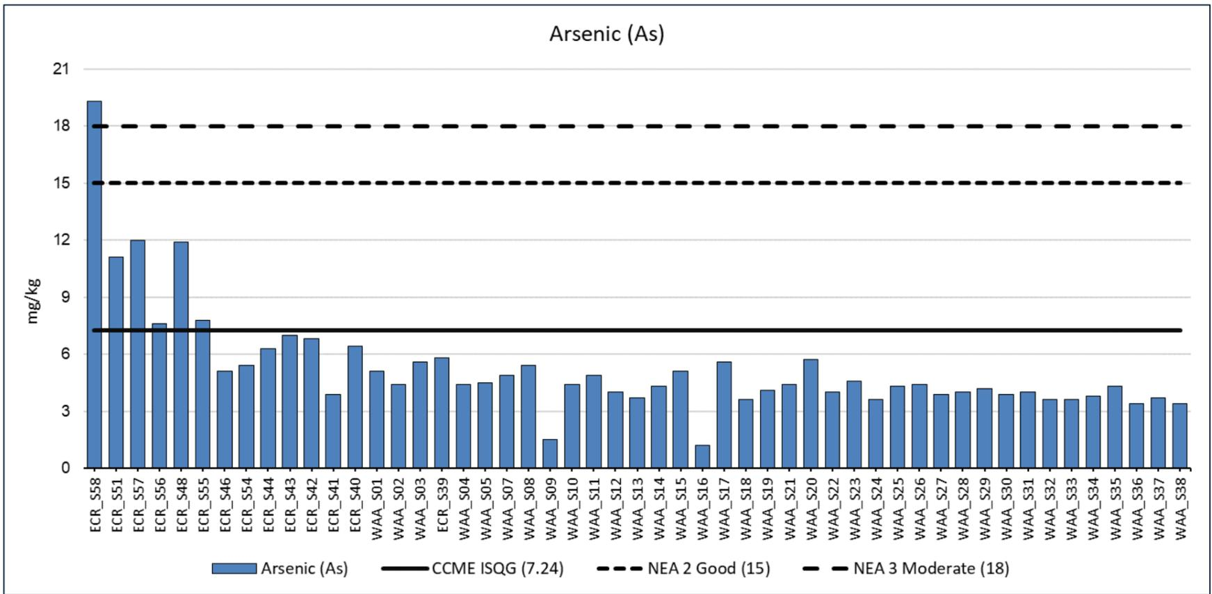
Figure 16 Arsenic (As) levels (mg/kg dry weight) from grab samples with threshold values, sorted by increasing easting.
