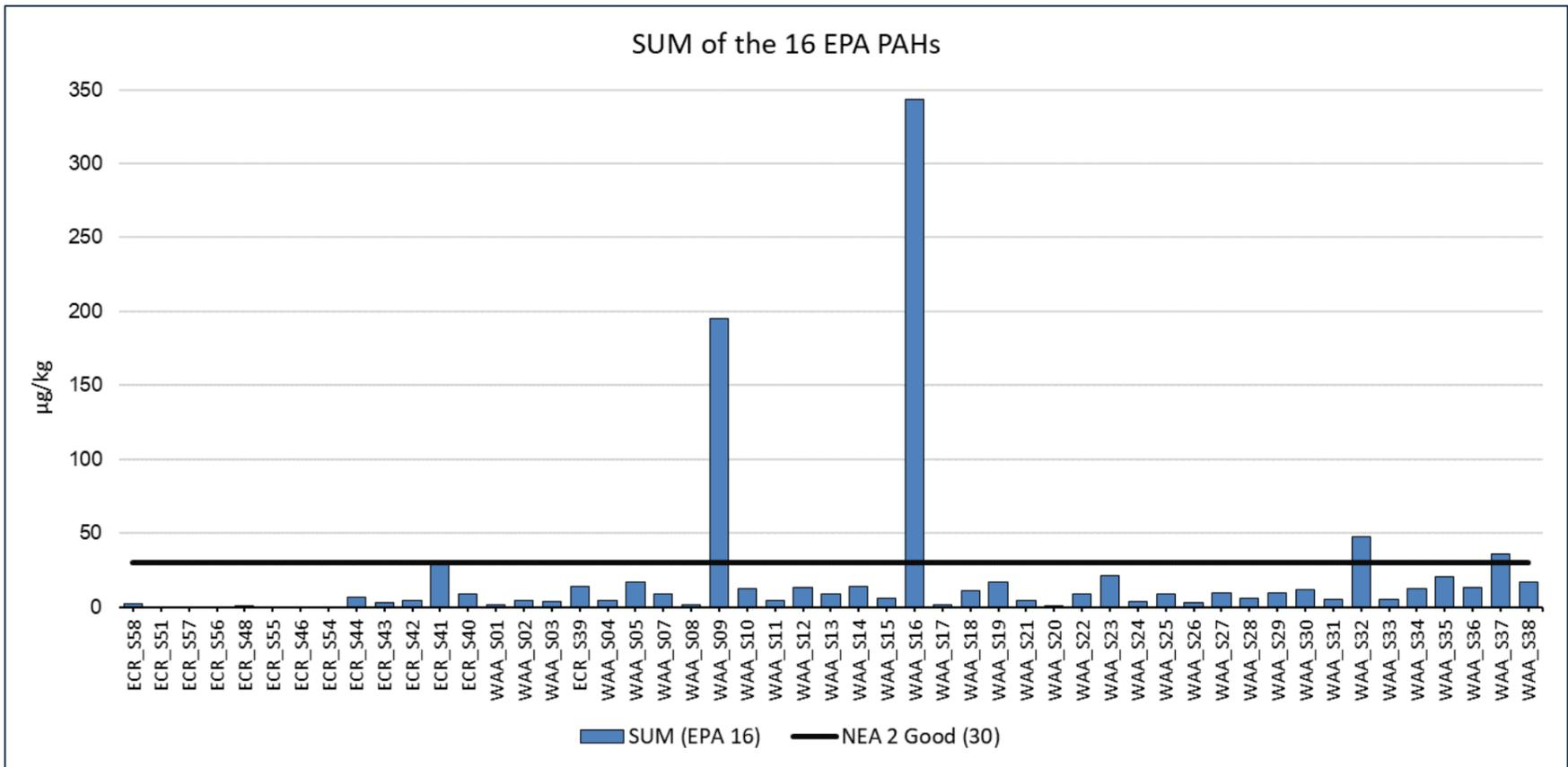
Figure 17 Levels of EPA 16 PAHs summarized (µg/kg) samples with threshold values, sorted by increasing easting.
