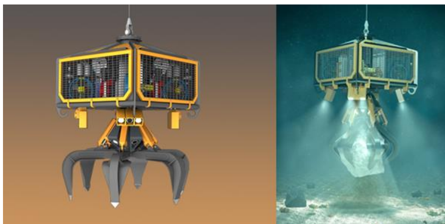
Figure 5.4: Example machinery for boulder clearance pre-cable lay.
